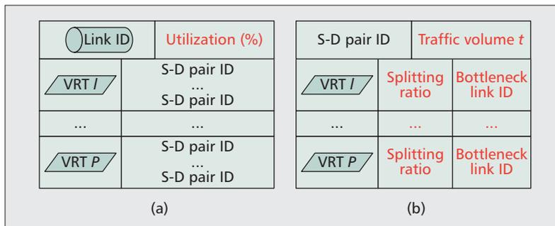
Figure 4. Traffic engineering information base structure: a) entry structure of LL; and b) entry structure of SDPL.
