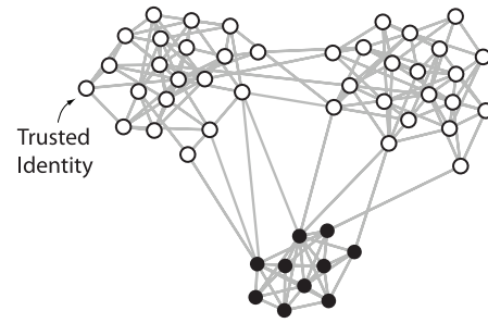
Fig. 3. Non-Sybils are hollow and Sybils filled. The trusted identity cannot distinguish between the non-Sybil community and the Sybil community.
