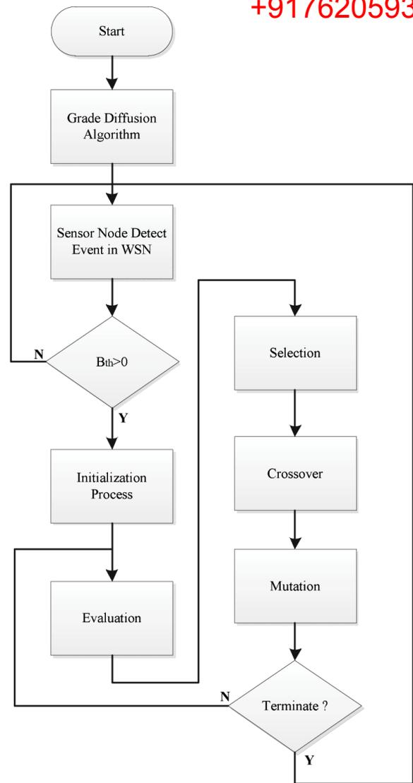
Fig. 3. Fault node recovery algorithm flow chart.
