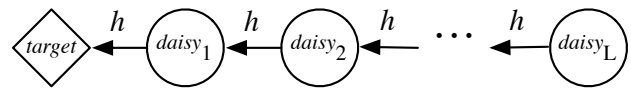
Fig. 5. Given daisy_i it is easy to verify the freshness of the blacklist by applying h i times to obtain target . Only the NM can compute the next daisy_{i+1} in the chain.
