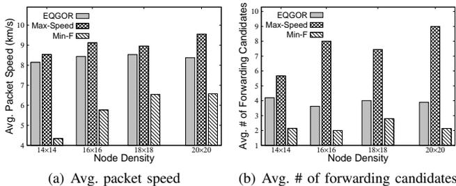
Fig. 4. Comparison with two extreme solutions in terms of the packet speed and number of forwarding candidates under different node densities
