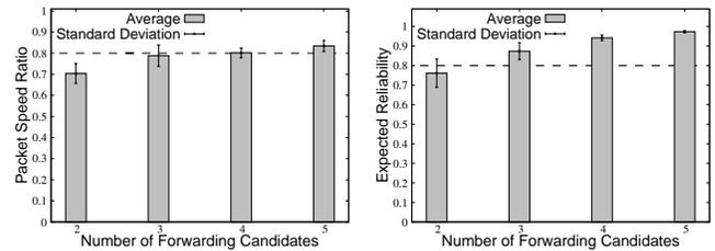
(a) Ratio of the expected one hop packet speed to the optimal value (b) The expected one hop reliability
