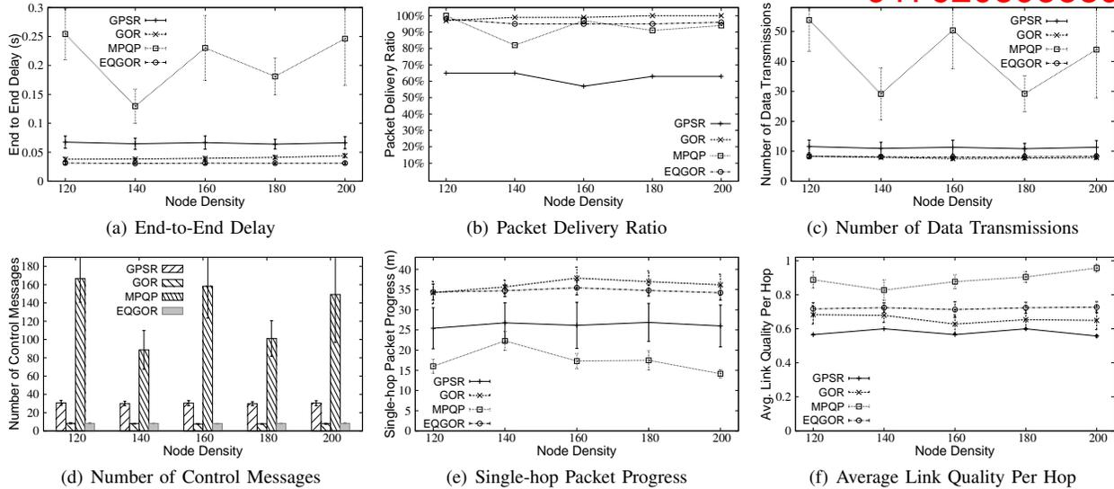
Fig. 5. Impact of the node density, the end-to-end reliability is set 0.95, and only the successful end-to-end transmissions are counted.
