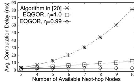
Fig. 9. Average computation delay measurement on the MicaZ node
