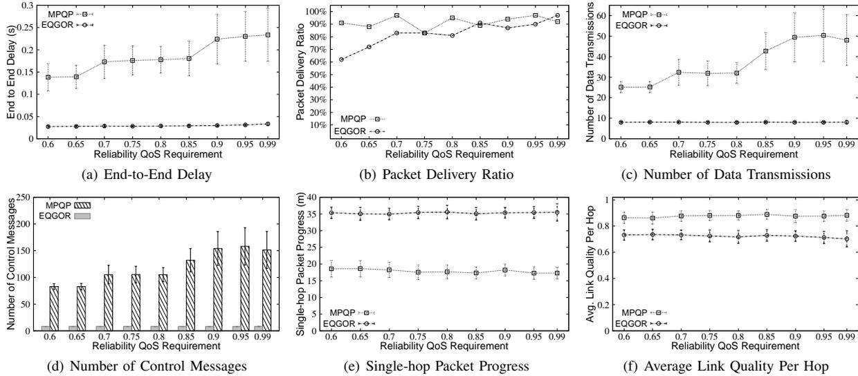
Fig. 7. Impact of the reliability QoS requirement in 160-node random network, and only the successful end-to-end transmissions are counted.
